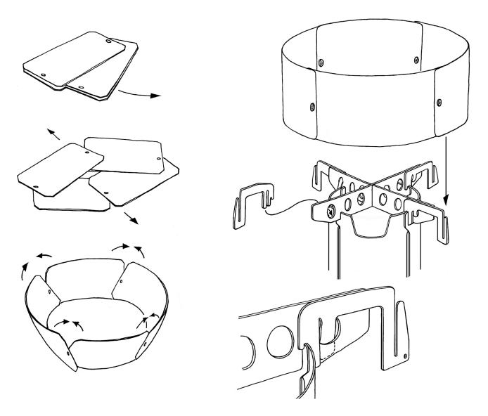
The windscreen made of four aluminum sheets, these are fixed with metal brackets attached to the FIBI-Stove.
